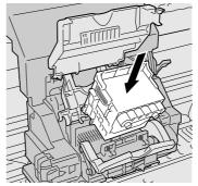
**13** Lower the printhead lock cover toward you to lock the printhead in place.
